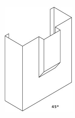
**NOTE:** Stops are fully and continuously welded, ground smooth, refinished and repolished to a #4 finish.
